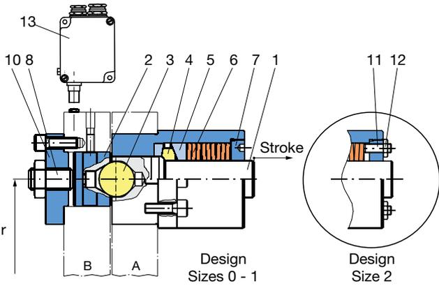
Fig. 1: EAS®-element engaged
