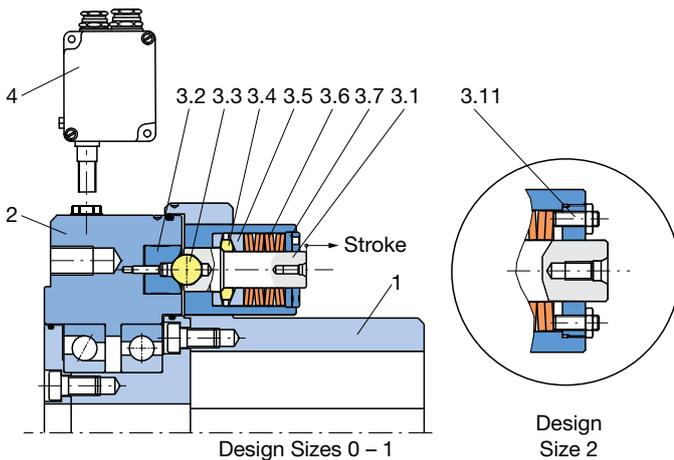
Fig. 1: EAS®-element clutch engaged
